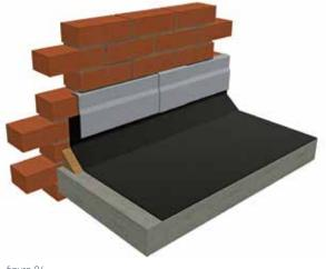
figure 04 flashing to a flat roof upstand
