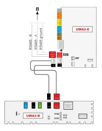
Modbus connecting (A) with a standard Brink HRA with only fitted the PCB UWA2-B
