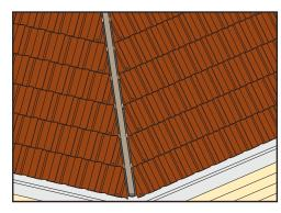
5. Starting at the eave, roll out the vent roll centrally along the entirety of the hip. Neatly trim the roll at the eave and at the ridge allowing the roll to overlap the apex by 100mm. Fix the roll at 450mm intervals to the hip batten using felt nails.
