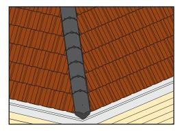
10. At the ridge/hip junction, ensure the last tile in the run is a full tile by cutting the previous tile down in length. Mitre cut the three tiles at the junction to fit neatly together, drill and secure them in place with the screws supplied. If required a small bed of mortar can be used to support the mitred tiles. Seal the mitred joints with a suitable roofing waterproof sealant.
