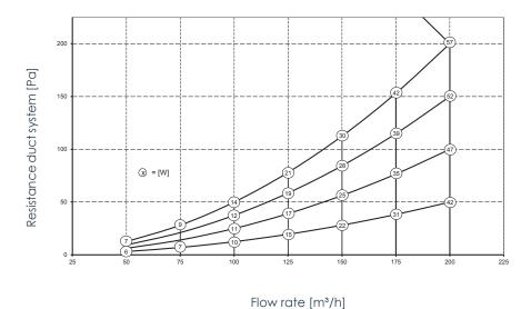
Note that the values circled in the graph are the power used ('Watts per fan)
