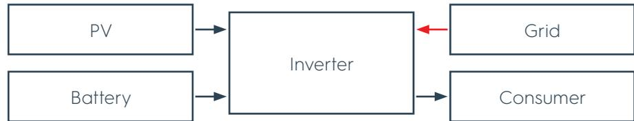
**Figure 21** Solar energy and battery not sufficient, additional energy from the grid
