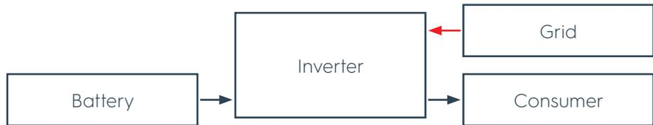
**Figure 29** Energy from the battery not sufficient, additional energy from the grid
