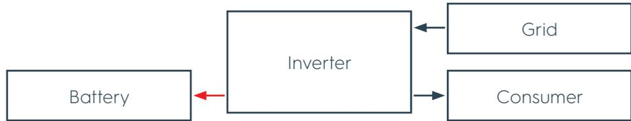
**Figure 27** Energy for battery charging from the grid
