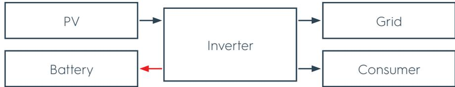
**Figure 30** Sufficient solar energy, surplus energy for consumers and into the grid
